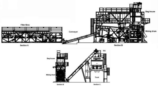
Figure 8 - conceptual layout of module plant
