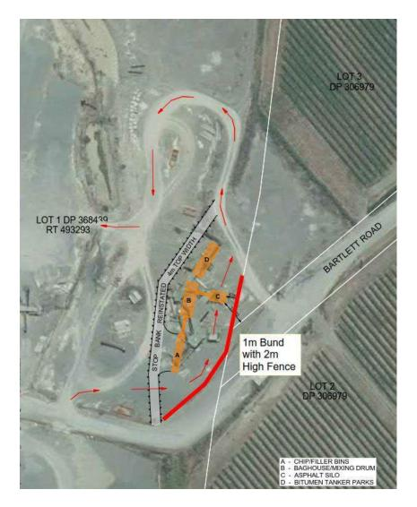
Figure 3. 3m Acoustic Barrier (red line)
