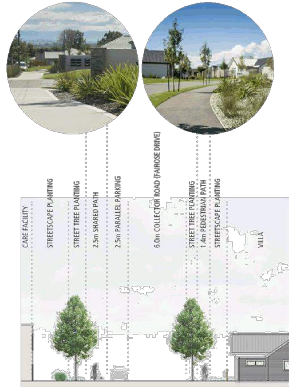
6 METRE COLLECTOR ROAD (FAIROSE DRIVE) | SECTION D-D
