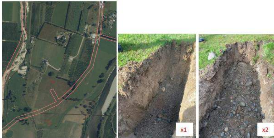
Figure 1 shows the location of interest and the two sites that were inspected during the field visit. A visual assessment found that the topsoil horizon was deeper at soil pit 1 (site x1) than found at pit 2 (x2). The soil in pit 2 also comprises of more sand and gravel than the soil in pit 1.
