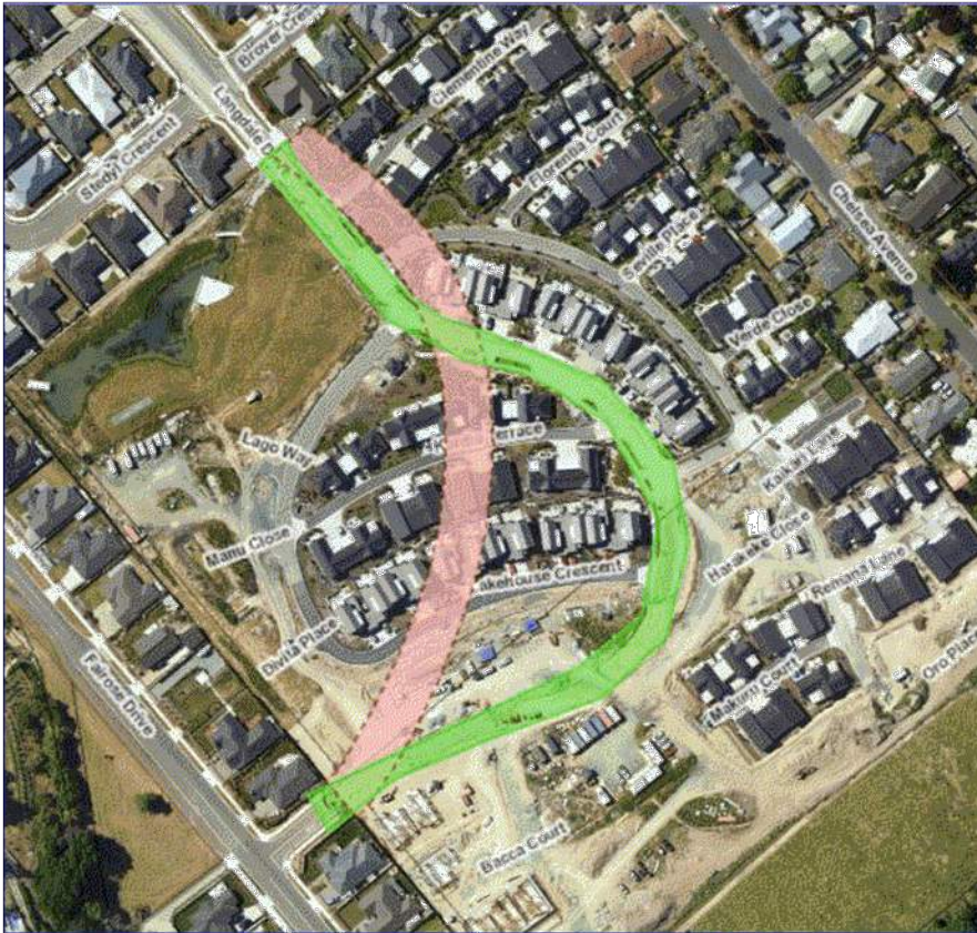
Plan of existing Olive Estate road (green) and TRMP Indicative road (pink)
