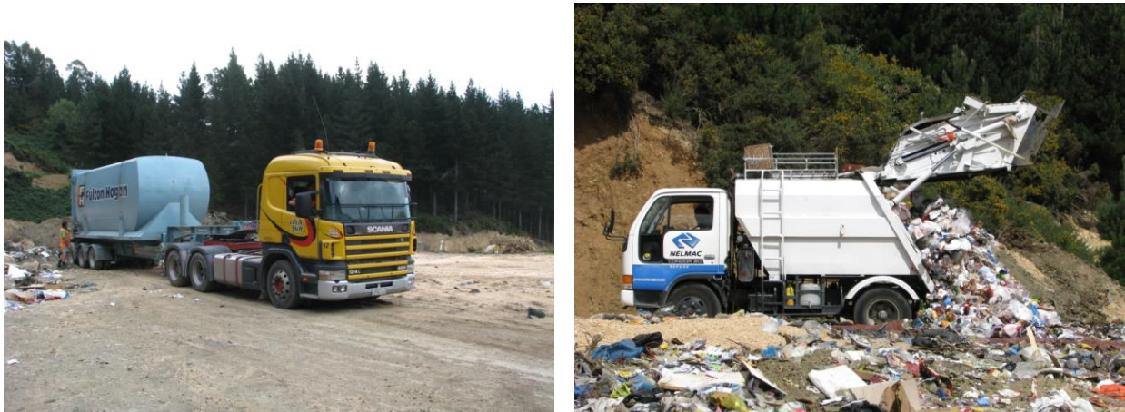
Figure 4-3: A typical compactor bin and compactor truck arriving at York Valley Landfill
