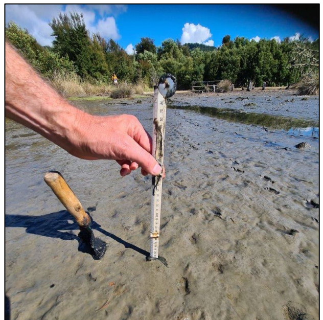
The depth of the anoxic muddy sediments was approximately 50-250mm deep, and overlaid a firm soil base in which the root mass of former vegetation is still present.
