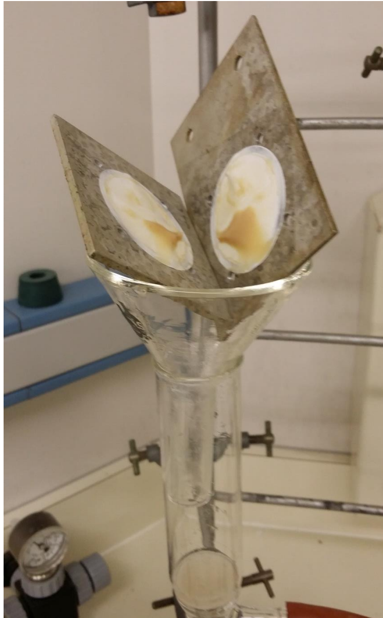
Figure 2-2: POCIS sampler being prepared for extraction. Note the brown paste is the POCIS sorbent and the white circular patches are the two membranes.
