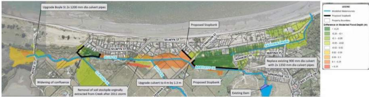
Figure 2. Flood level difference map comparing the present day scenario (baseline) with the modelled flood levels after the proposed mitigation measures as identified in call-out bubbles are complete.
