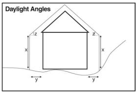
angle across the site depending on the direction the boundary faces. For example, the angle is 45 degrees for north-facing boundaries, 35 degrees for east and west-facing boundaries and 25 degrees for south-facing boundaries. No building can project beyond the daylight admission angles, although the TRMP includes exceptions for gable ends and alternatives for a site on a south-facing slope.
