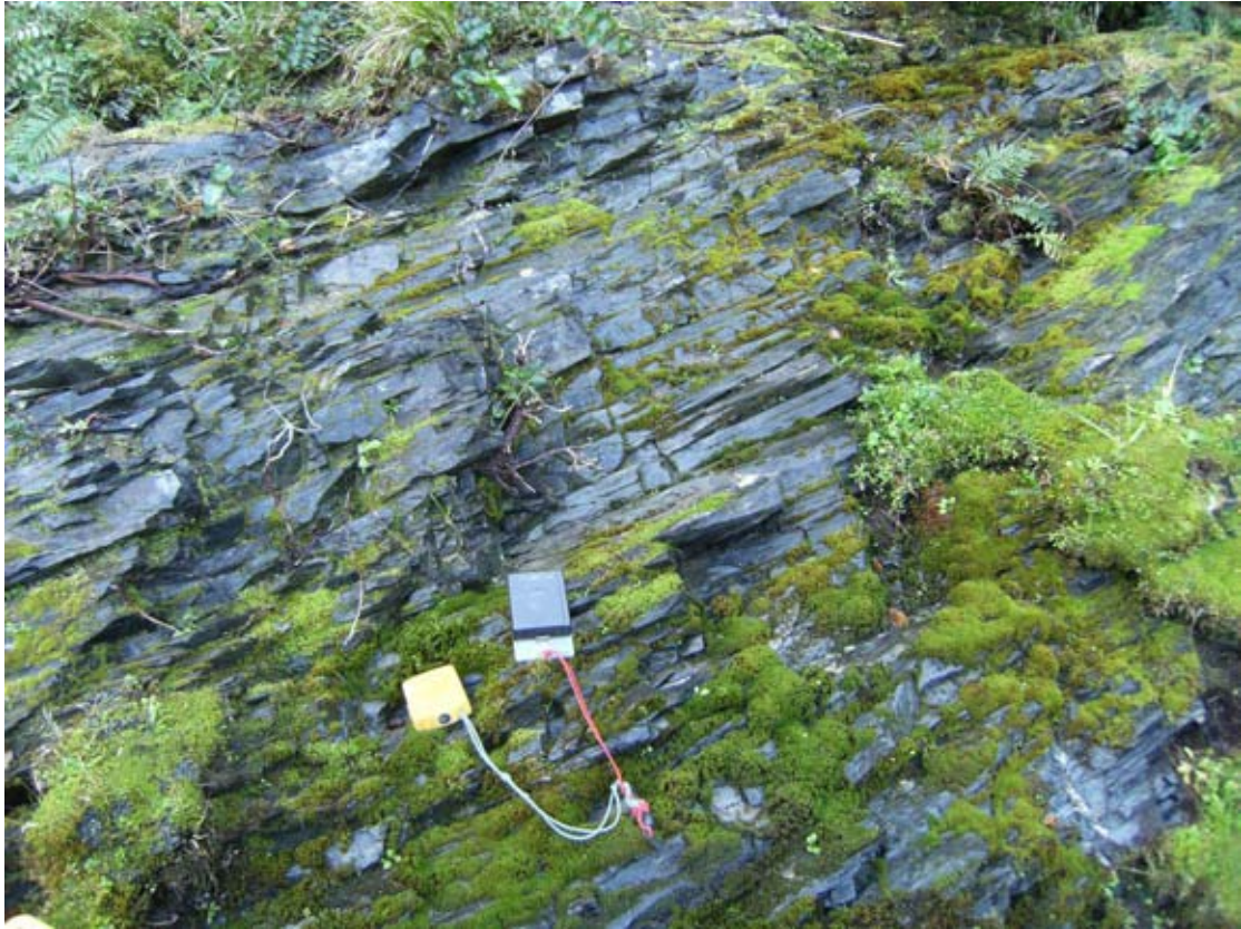
Photo 9: Laminated greywacke in river exposure in dam foundation
