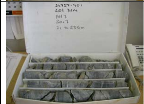
Drillhole 7: Core Boxes 4-7
