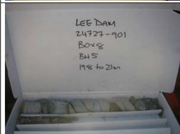
Drillhole 5 Core Boxes 5-8
