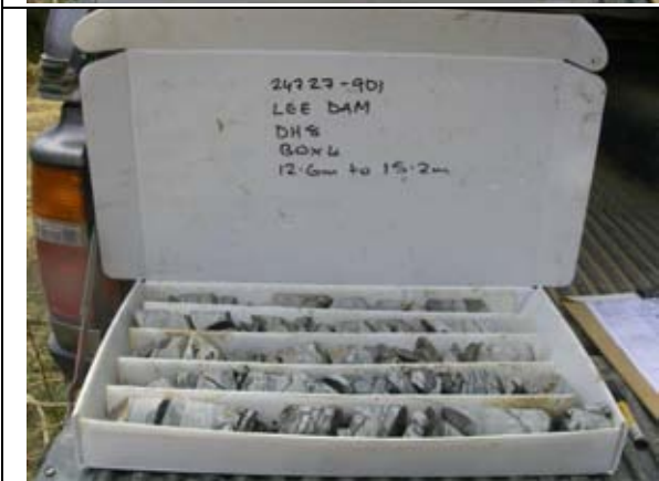
Drillhole 8: Core Boxes 1 - 4
