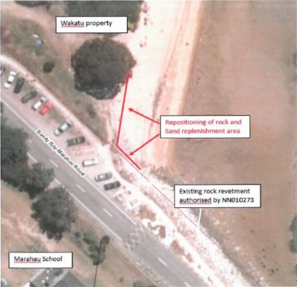
Figure 16: Location of the proposed sand replenishment works.
