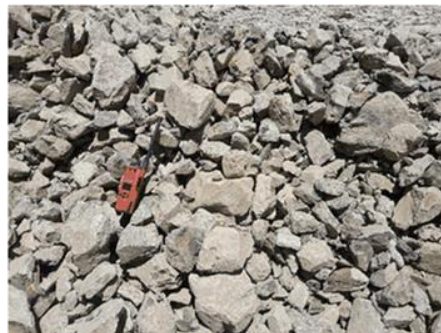
Figure 28: Unsuitable indigenous rock breaking down Figure 29: Imported suitable drainage material
