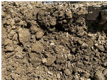
Figure 28: Unsuitable indigenous rock breaking down Figure 29: Imported suitable drainage material
