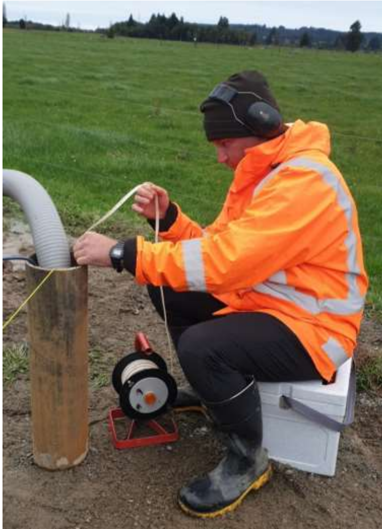
WWD 24431 – Swamp Road. Photo showing the water level being read during a pumped aquifer test.
