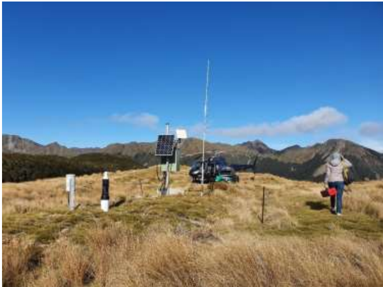
Wangapeka at Biggs Tops Rain Gauge communicates via satellite telemetry. It records highest rainfall during events with winds from a north-westerly direction. The site has operated since 1989.
