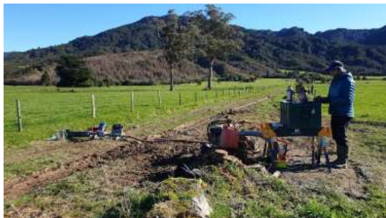
WWD 24433 – Kaituna. Photo showing the bore undergoing a pumped aquifer test
