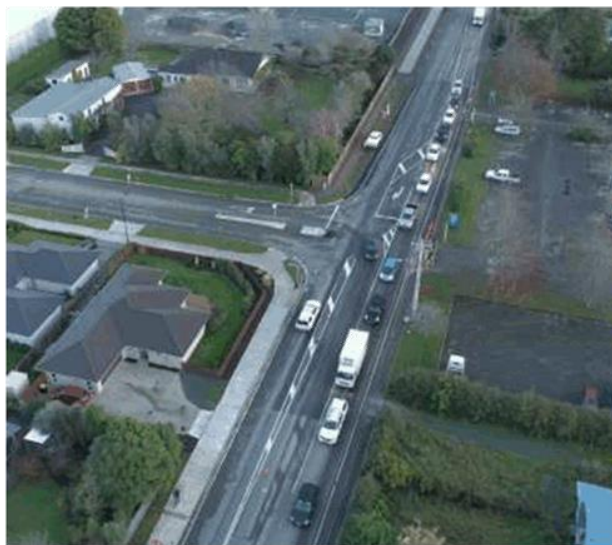
Lower Queen Street/Berryfield Drive new intersection layout
