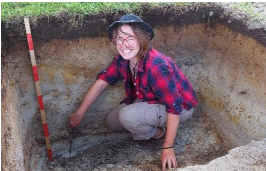
This is Anne in her happy place after digging a 1.8 m x 1.2 m x 1.0 m soil profile (Mottled Orthic Allophanic soil)
