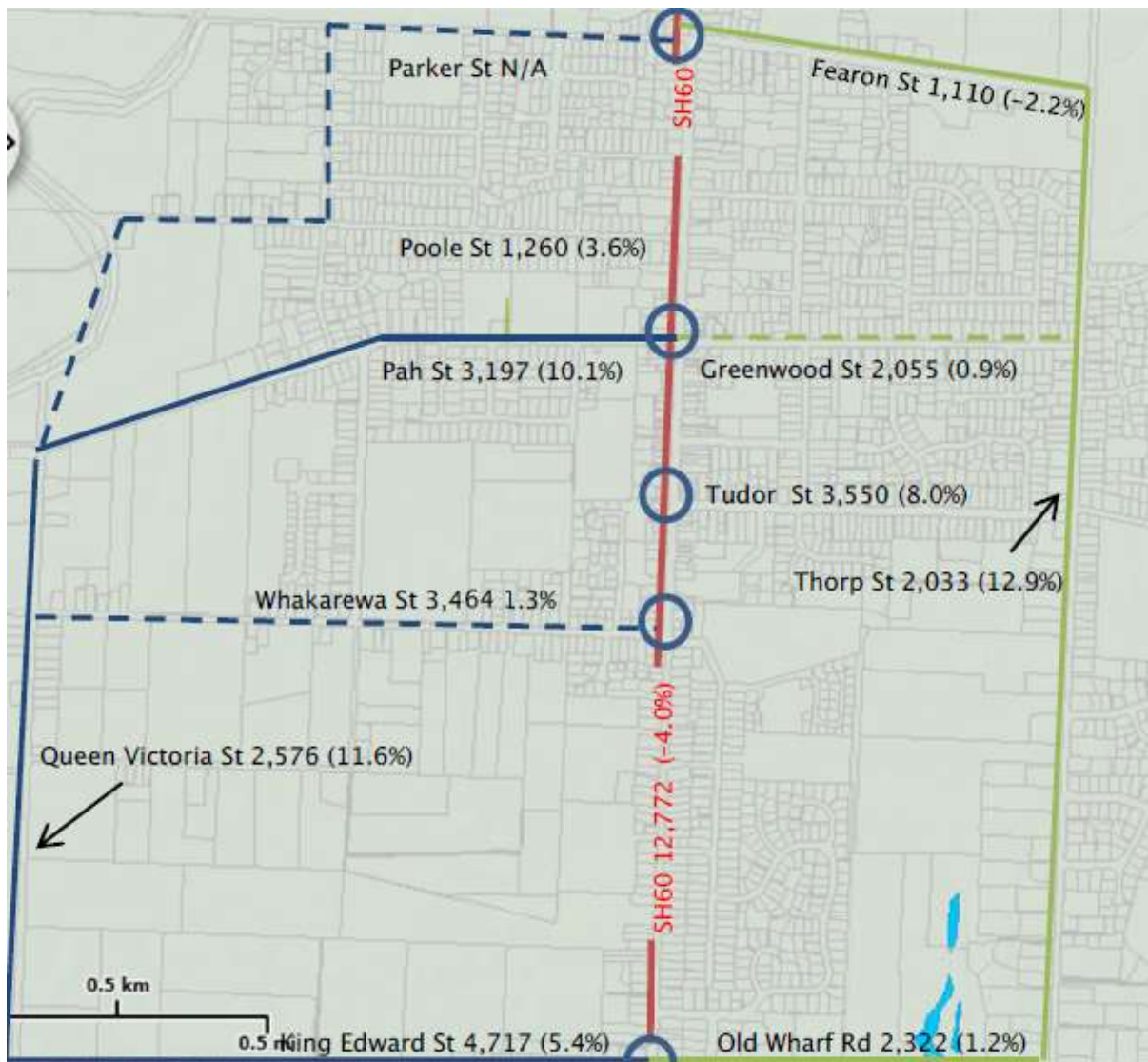
Figure 33: Motueka Traffic Volumes and Growth on Alternative Routes from SH60 Motueka Strategic Case, NZTA
