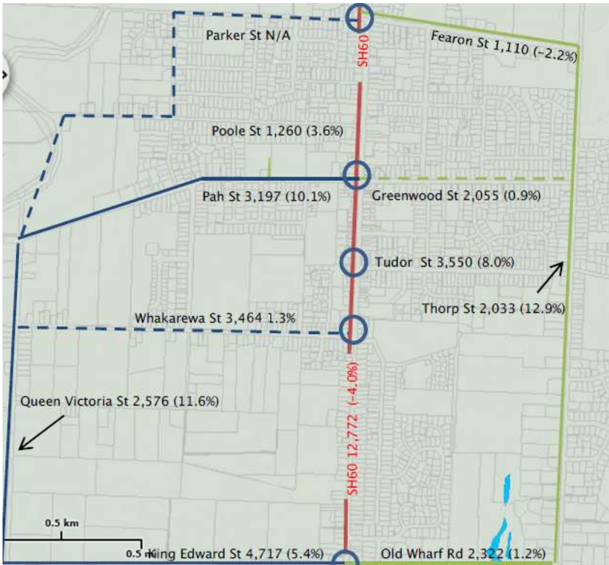
Figure 32: Motueka Traffic Volumes and Growth on Alternative Routes from SH60 Motueka Strategic Case, NZTA
