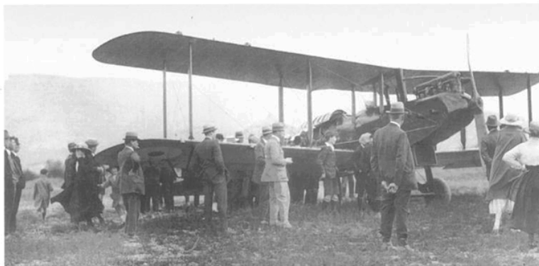
The de Havilland DH9 attracted significant attention and Hawker was keen for local people to feel confident about a flight. The aircraft retains its Royal Air Force markings and the fuselage canopy is open ready for the next passengers. Note the prominent radiator below the Armstrong Siddeley Puma engine of 265hp. VIA DAVID MILLER
