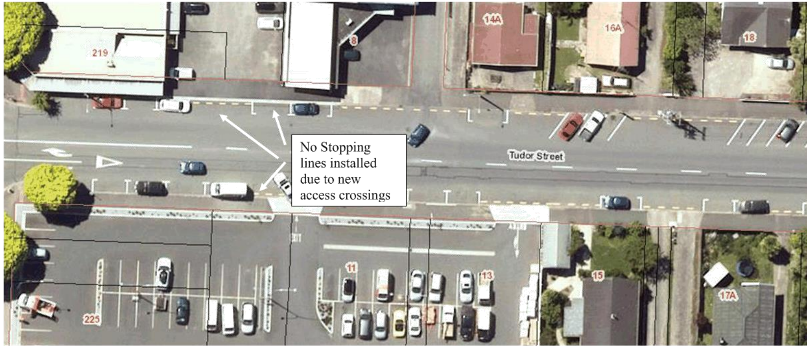
Tudor Street – Removal of various Park Limit lines and marking of new lines including removal of some No Stopping lines due to new access crossings
