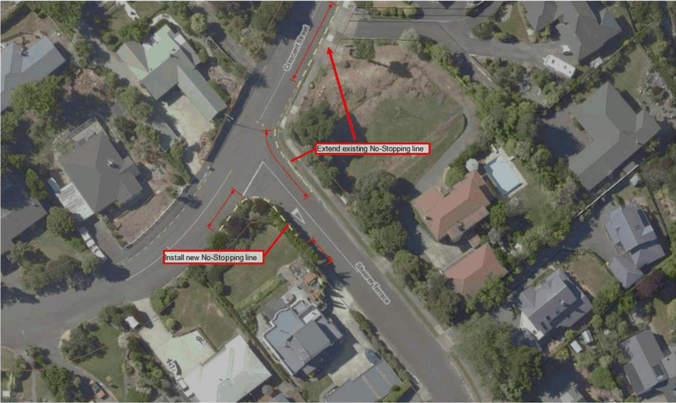
Crescent Street at Shearer Terrace – No Stopping lines
