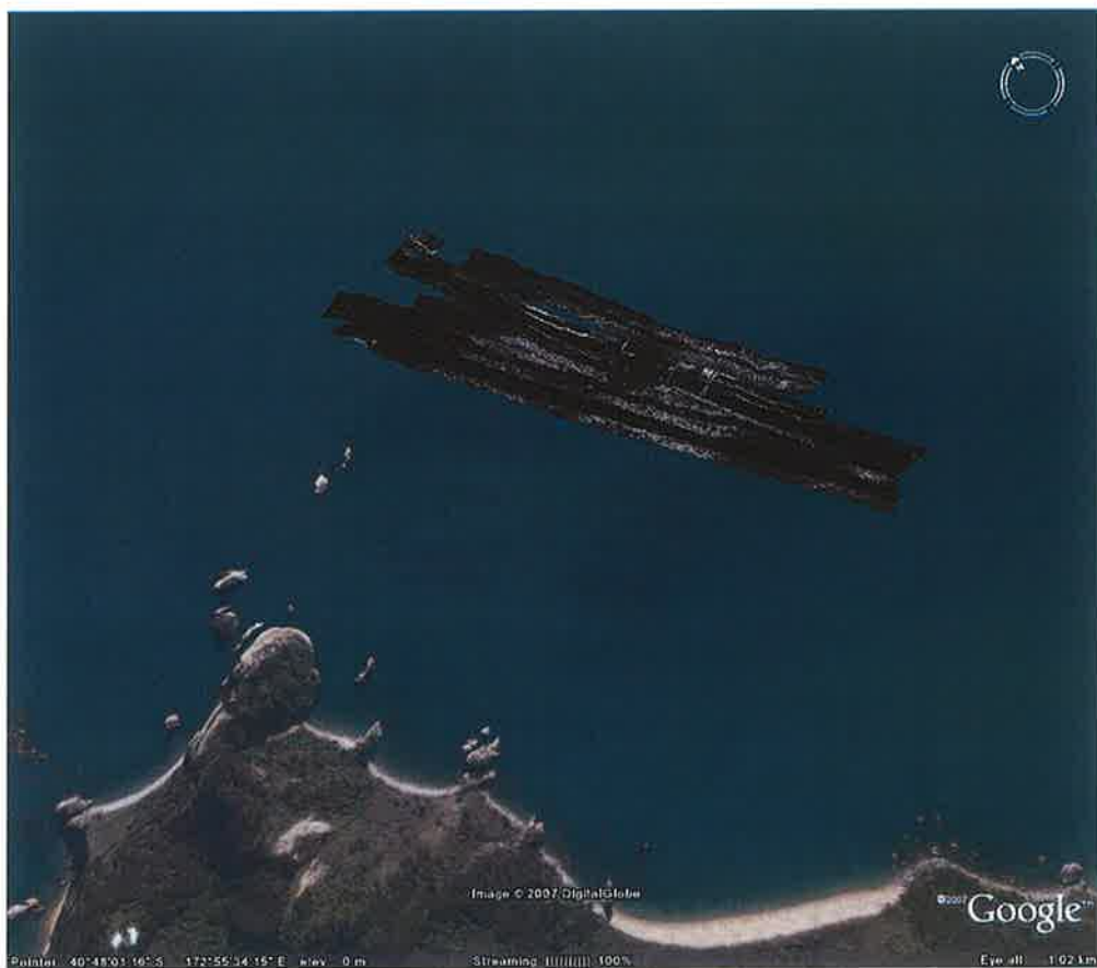
Figure 7. Geo-referenced side-scan sonar transects overlaid on a Google Earth image of the spat farms at Wainui Bay. The surface structures of spat farms inshore of Pe30 and Pe31 are clearly visible, as is highly reflective material directly beneath P30 and Pe31.
