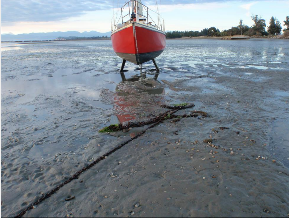
Plate 3. Traditional swing mooring in Moutere Inlet. Note keel settlement depressions.
