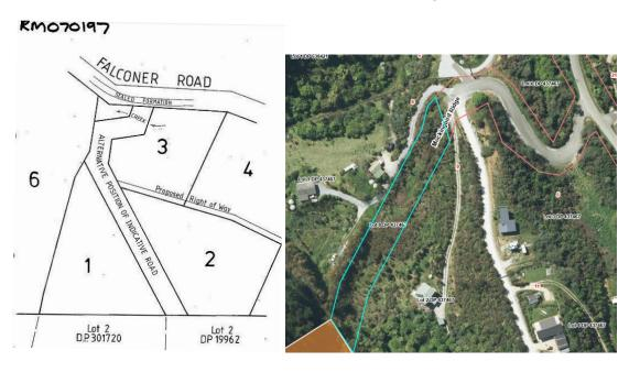
It is likely a complying road can be formed along this alignment to Haile Lane (via existing indicative roads) but will require cuts and fills and a culvert crossing.
