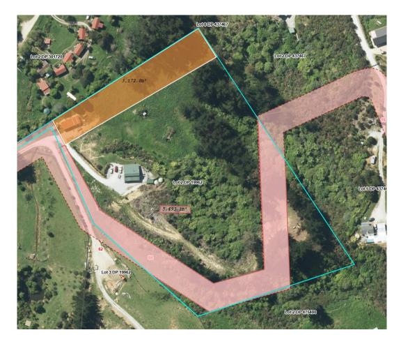
It is noted there is less land area taken up on the submitters land for the new proposed indicative road alignment, i.e., existing is 5,493m2 (pink above) and proposed is 3,172m2 (orange above). It is noted that a shed would need to be removed with the proposed alignment and that a future road at the front of the property has a different impact than one at the back.
