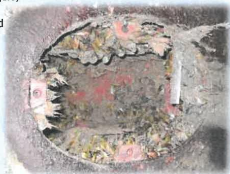
Clogged sea chest. Photo: Cawthron Institute.
