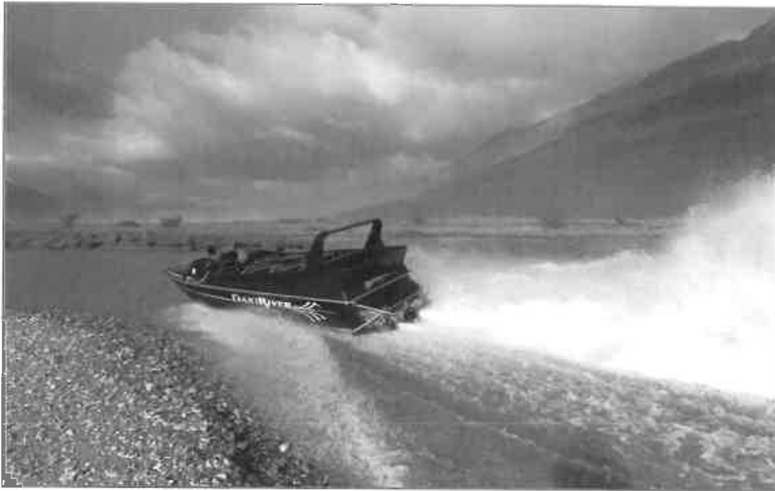
Figure 11. Dart River Safaris DRS10 twin V8 engine 7.1 m jet boat used in the bank erosion trials (2013 May 25)
