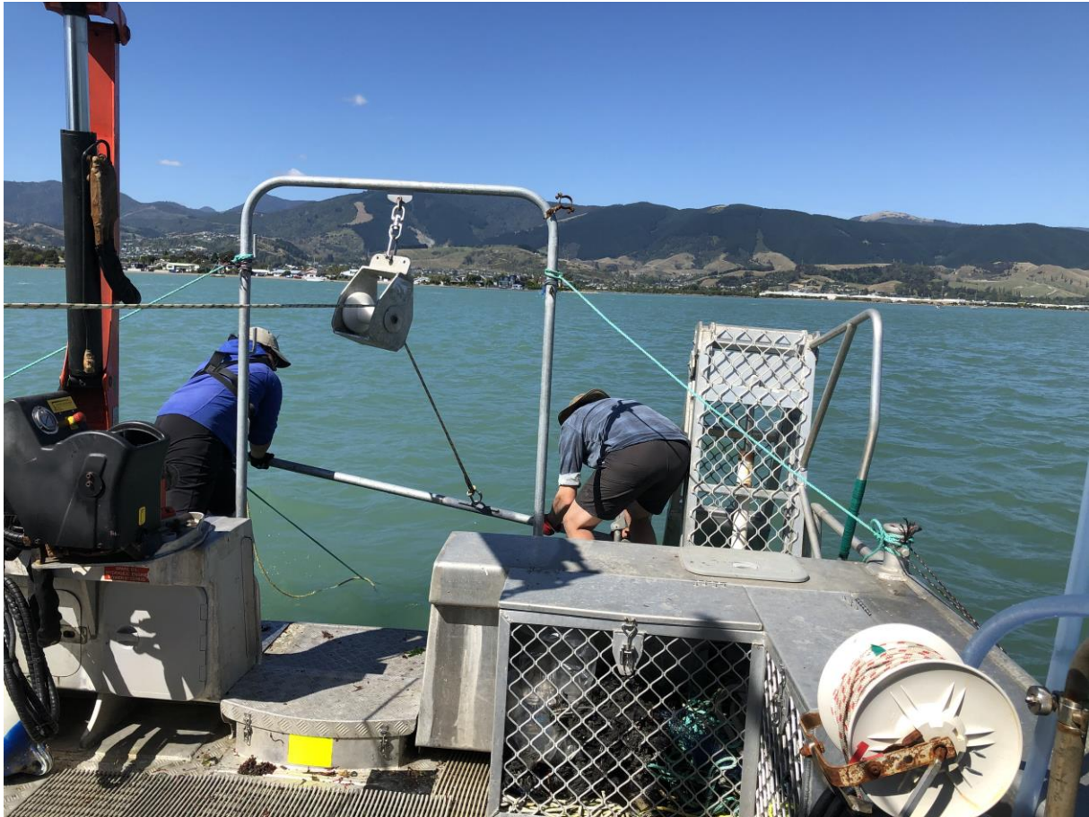
Figure 8: The beam trawl being deployed. The three-metre bar is being handled by two field staff, with the net itself being submerged behind the survey vessel.
