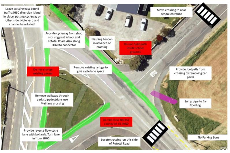
New pedestrian crossing for Commercial Street South of Rototai intersection Flashing beacon in advance of crossing
