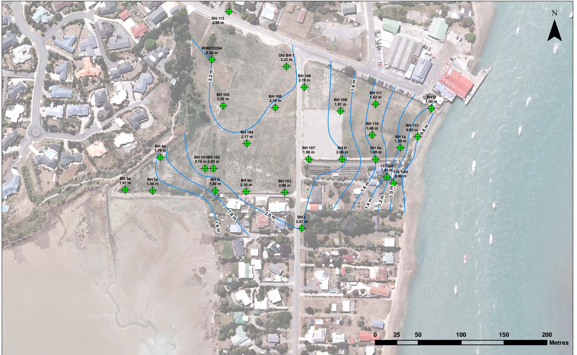
Figure 11 : Groundwater levels and contours on 9/02/10
