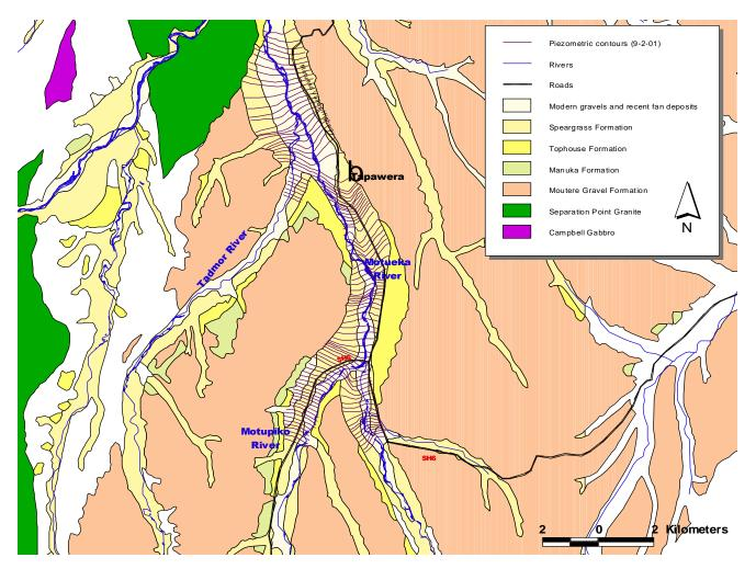
Figure 6: Piezometric map showing groundwater flow patterns in Upper Motueka February 2002
