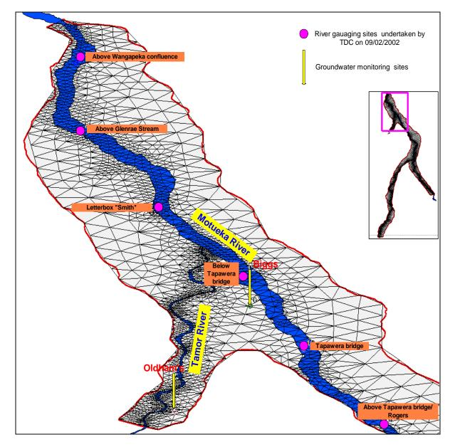
**Figure 1** Close up two-dimensional view of the Upper Motueka groundwater model domain with aquifer discretization and a finite element mesh. Total area of model domain is shown in inset box. The blue area is river channel. N.B. the finer mesh immediately adjacent to the river channel.
