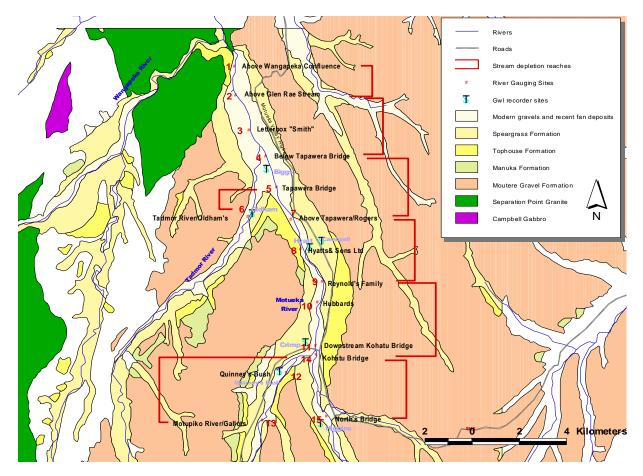
Figure 7: Stretches of Motueka Rivers used in stream depletion calculations
