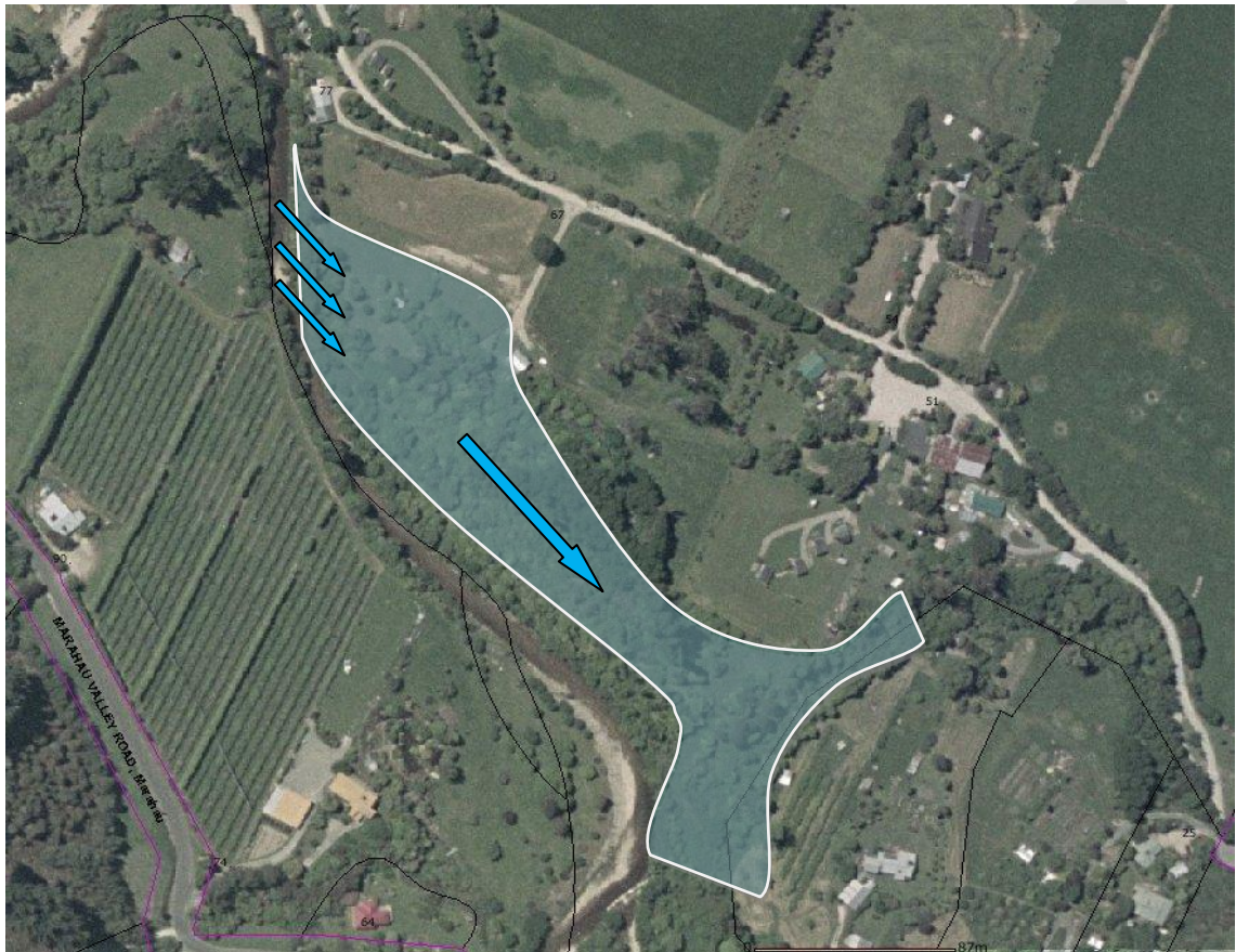
Figure 1: Estimated flood area based on walkover and observation of flotsam
