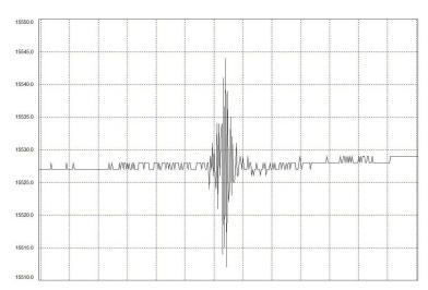
Each vertical square is 5mm change in water level, and each horizontal square is 5 minutes in time.
