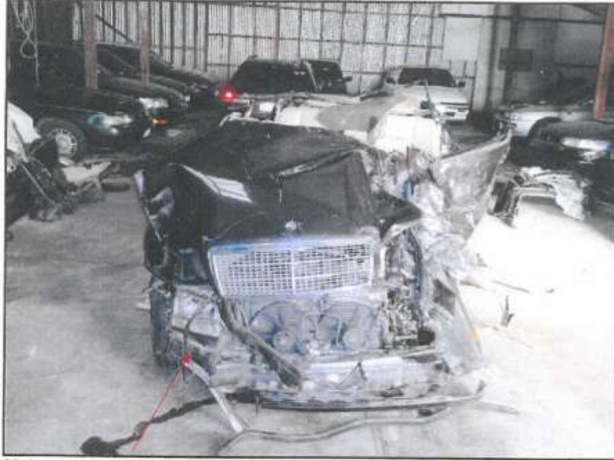
Note: secondary damage caused by impact with tree.
