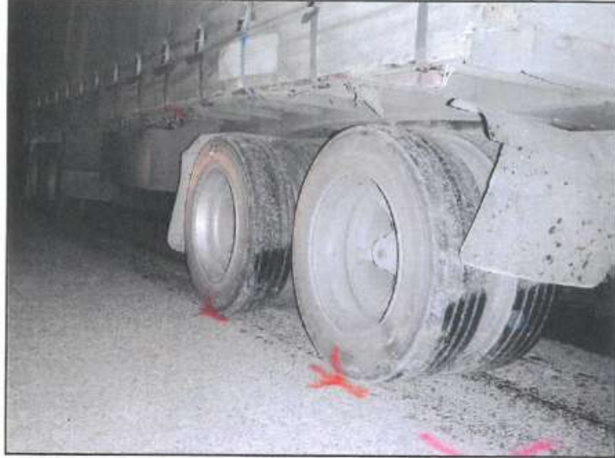
View of trailer tyres showing signs of wheel lock-up (taken in situ).
