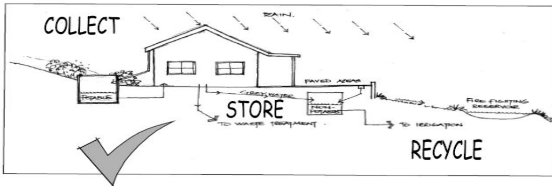
Figure 12 – On-site water storage, efficient use and re-cycling
