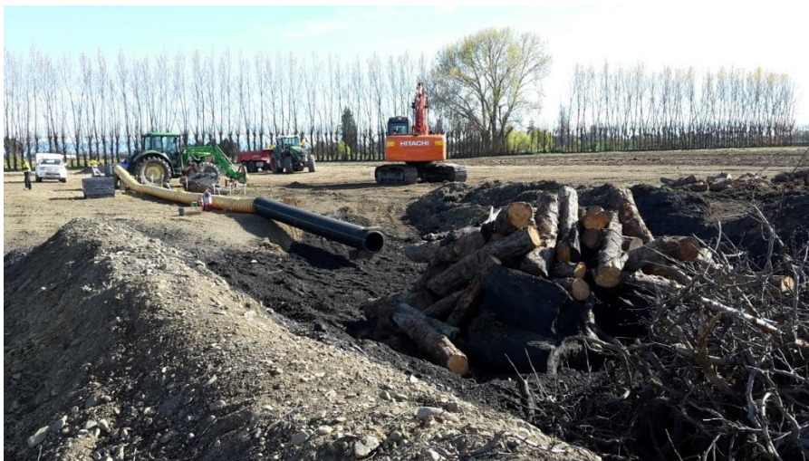
Photo 5: The setup of the outdoor burning trial – a tractor mounted fan attached to a pipe which blows air into the base of the fire, located in a trench.
