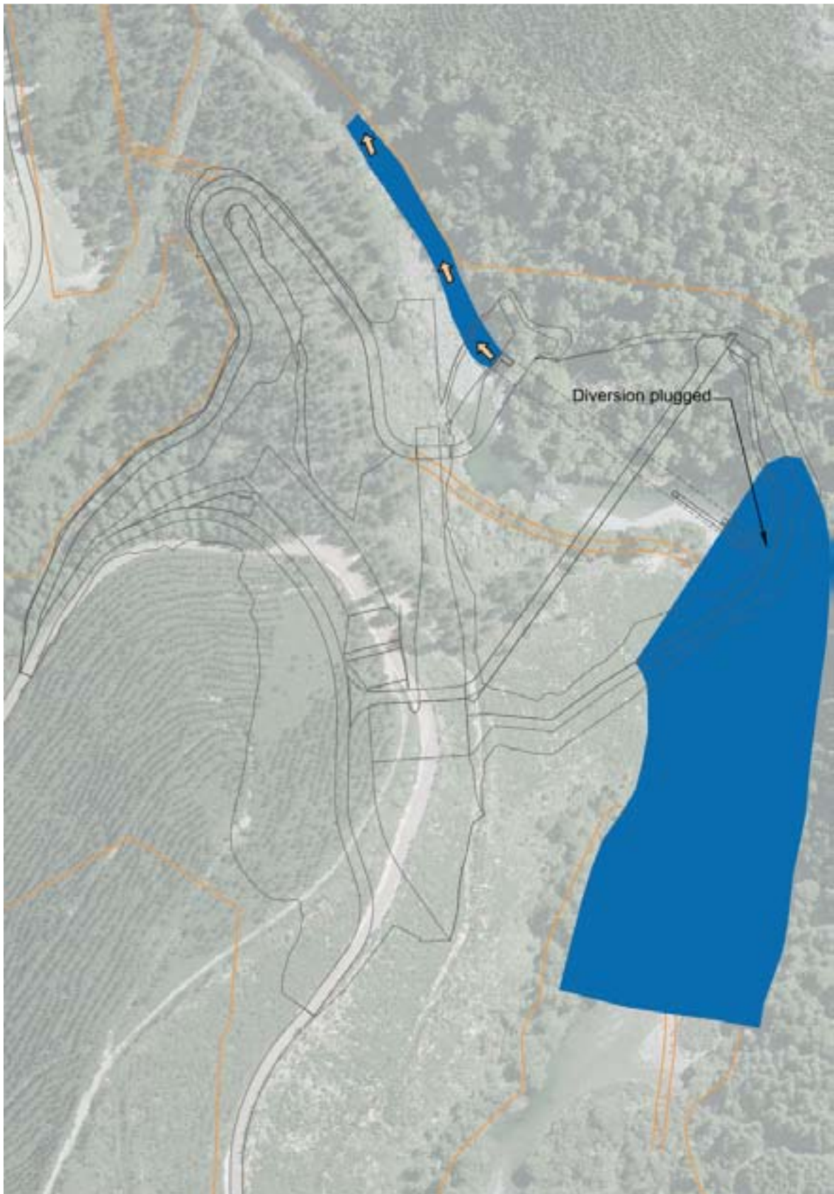
Figure 12-16: Sketch of Stage 7 of construction
