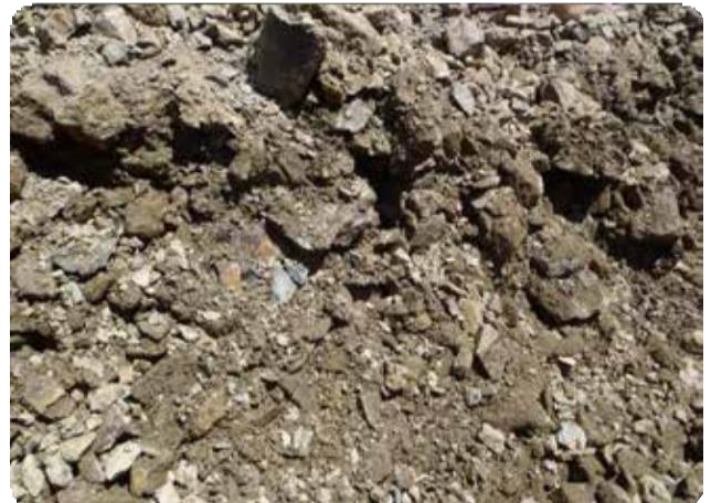
Not free draining rock encountered.
